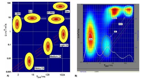
Figure 4 A) schematic D-T2 map and B) Real data derived D-T2int showing heavy oil spot, clay bound water (cbw), movable water volume (bvmw)and water based mud filtrate(wbmf) from [1].
