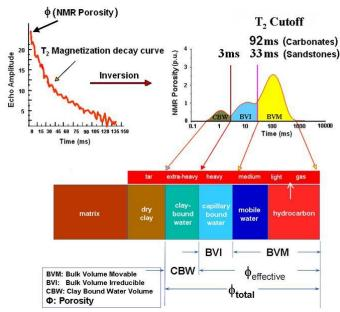
Figure 1 1D-NMR porosity model: Cut-off partition of T<sub>2</sub> spectrum
