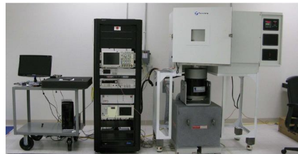
Figure 4. The dynamic test station for the Fiber Optic Seismic Sensors (FOSS). This test station can test the sensor at both low and high temperatures.
