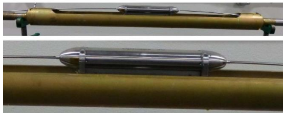
Figure 12a. The Sensor Pod installed into a Sensor Pod Housing.
